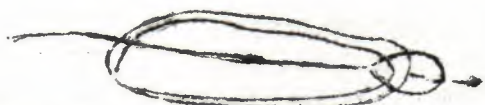
Pass loop over end of shock cord & pull shock cord through. The two are now firmly attached to each other.
